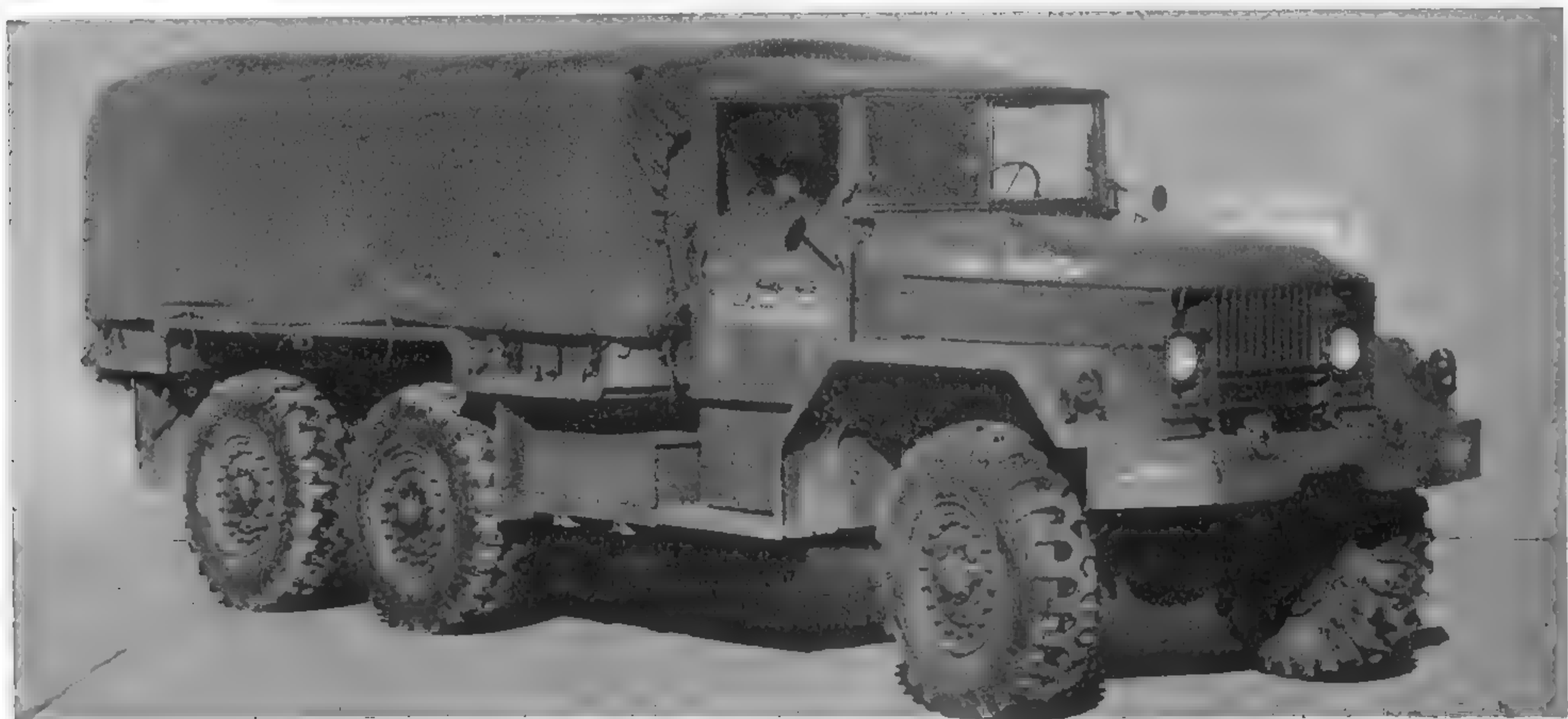
The XM41 was photographed for the Army Field Forces Board 2 prior to testing. The large 14.00-20 single tires all around and wheel well-type bed make these trucks stand out. (Photo courtesy of the Patton Museum)
